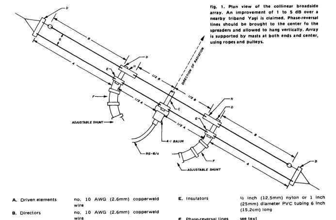
decided to match the antenna to 50 ohms by using a quarter-wave matching section according to the wellknown relationship
